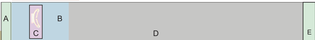
A: Adhesive strip B: Absorbent wound pad C: Open 'C' shape clip D: Main Bandage E: End anchor
